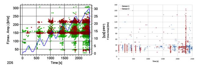
Figure 5 Peak frequency vs Time for (a) PZT sensor (b) FO sensor.
