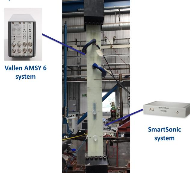
Figure 1. PZT and FO AE sensors attached to the specimen.
