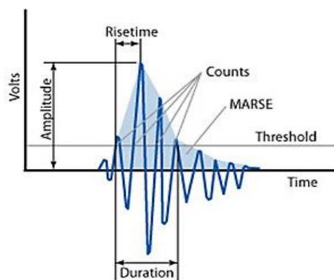
Figure 2. AE waveform parameters [2]
